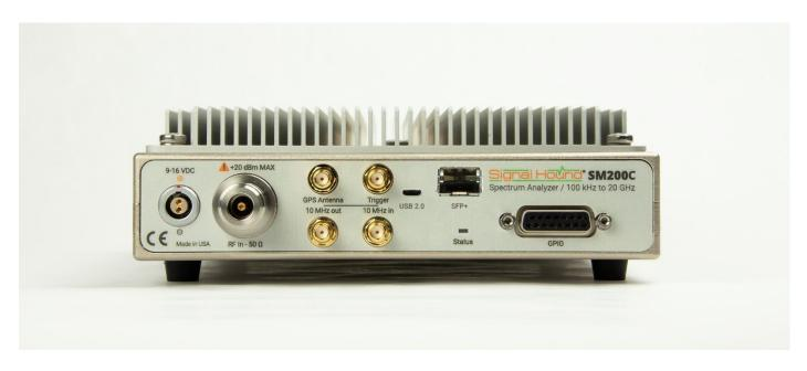
The SM200C is a high-performance spectrum analyzer and monitoring receiver with a 10 Gigabit Ethernet SFP+ port, which enables the SM200C to communicate with a PC over long distances using a fiber optic cable. Tuning from 100 kHz to 20GHz, the analyzer has 160 MHz of instantaneous streaming bandwidth (IBW), 110 dB of dynamic range, 1THz/sec sweep speed at 30kHz RBW (using Nuttall windowing), and phase noise performance that rivals even the most expensive spectrum analyzers on the market.
